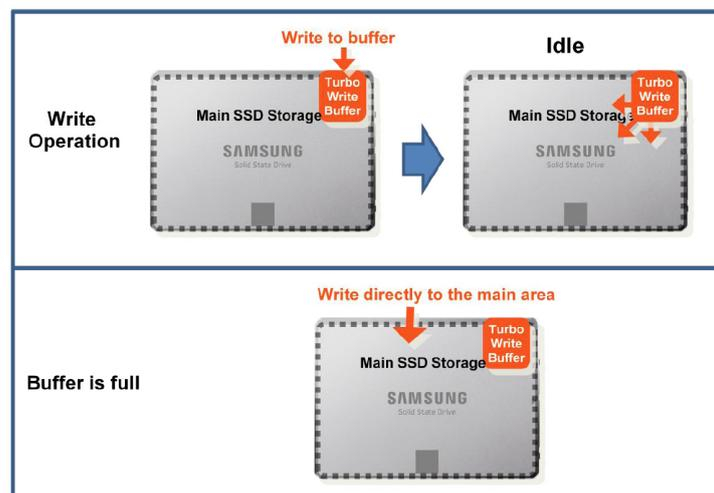
[Figure. 1] TurboWrite Technology algorithm
